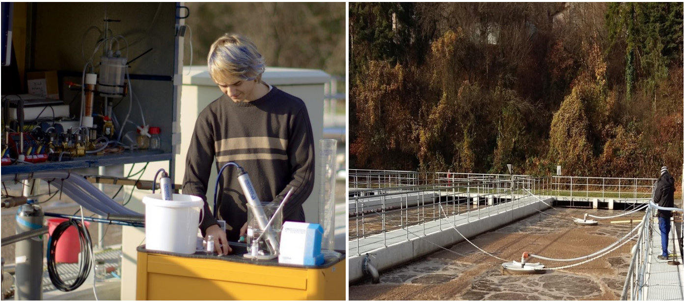
Fig. 2: Calibration of the sensors by Mr. Stefan Kühling. (Specialist for wastewater engineering at the WWTP Pforzheim)
