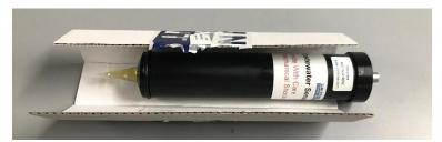
Place the Sensor Head in the cardboard protection sheet that came with the sensor. If this has been lost, another piece of cardboard may be used.
