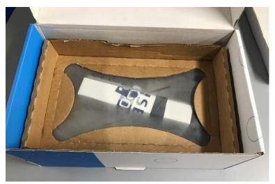
Place the second membrane insert with the membrane facing downwards. The Sensor Head must now be squeezed in between the two membranes.
