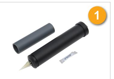
Together with the  $N_2O$  sensor head replacement you will find a small pack of lubricant for the O-rings on the sensor and housing. You also need the plastic tube you received with the system to change the  $N_2O$  sensor head.
