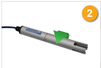
Unscrew the sensor body by holding on to the top (with the logo) and turn bottom part counterclockwise. Be careful when separating the two parts.
