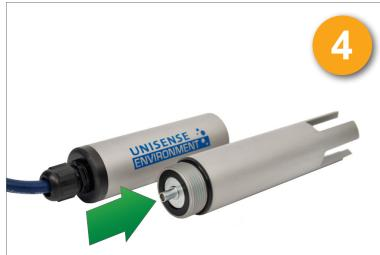
After inserting the new  $N_2O$  sensor head, assemble the sensor and connect it to the control box. When the sensor is connected to the control box let it stabilize overnight before proceeding with the calibration procedure.
