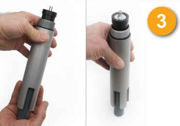
Use the plastic tube to push the old sensor head out of the sensor body. Next, apply grease to the two O-rings (one on the replacement sensor and one on the housing). You can now proceed to insert the new sensor in the housing!
