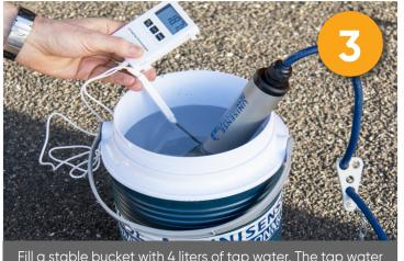
Fill a stable bucket with 4 liters of tap water. The tap water temperature should be close to that of the process water. Measure the temperature of the tap water and place the sensor in the bucket. Let the sensor signal stabilize.
