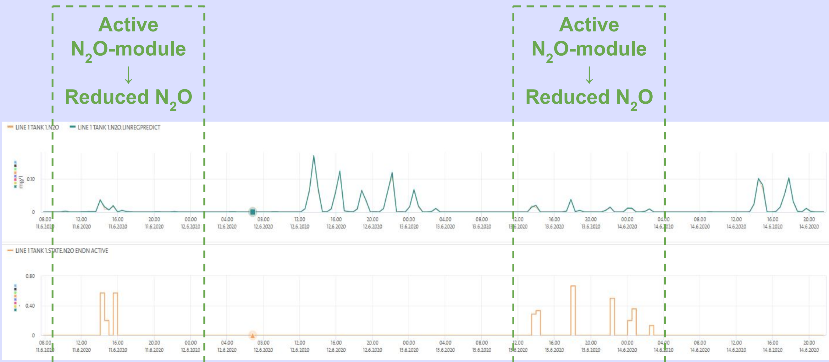
Example of N 2 O-reduction at Næstved WWTP. N 2 O is produced during the aerated phase due to the ND passway. To reduce N 2 O emission, the aerated phase is interrupt when N 2 O reach a certain setpoint. The N 2 O is quickly reduced when the O 2 is removed, showing sufficient COD for destruction of N 2 O. The activation of the N 2 O-module do not affect the NH 4 in the outlet.
