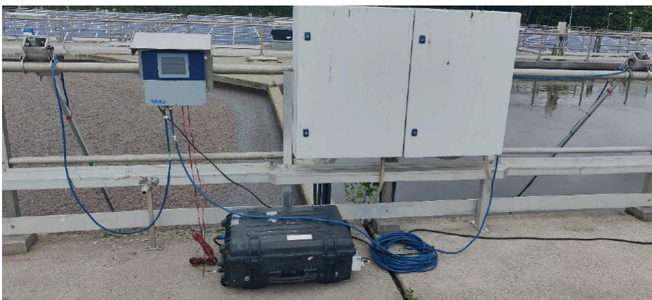
Figure 1: Sensor controller box, monitoring suitcase and equipment for sensor mounting used during the N_2O monitoring campaign.
