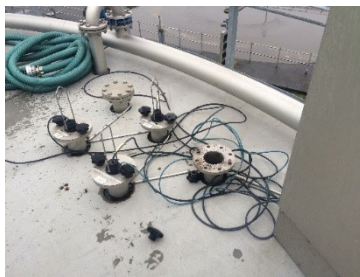
Cleaning of the \text{N}_2\text{O} Wastewater Sensor on top of the reject water tank at VandCenterSyd, Odense, Denmark
