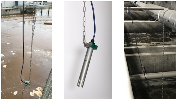
Solutions for mounting the sensor in wastewater.
