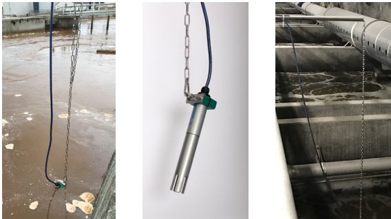
Solutions for mounting the sensor in wastewater.
