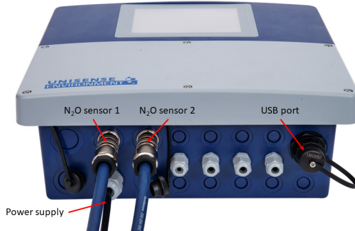
Back view of the N 2 O Wastewater Controller showing connections.
