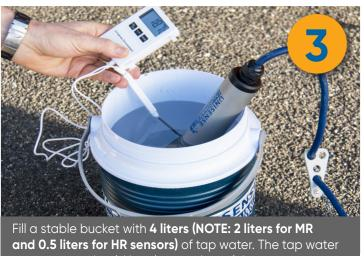
Fill a stable bucket with 4 liters (NOTE: 2 liters for MR and 0.5 liters for HR sensors) of tap water. The tap water temperature should be close to that of the process water. Measure the tap water temperature\* and place the sensor in the bucket. Let the sensor signal stabilize (min. 1 minute).
