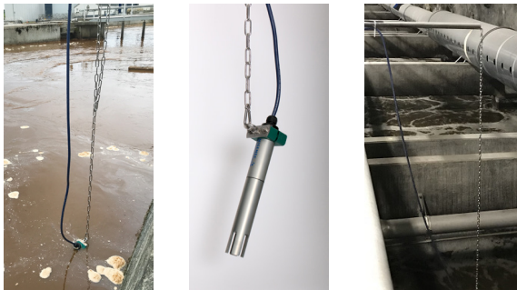
Solutions for mounting the sensor in wastewater.
