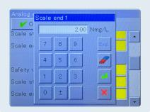
6. Enter the new max scale range that 20 mA corresponds to 10 mg  $N_2$ O-N/L is used here.
