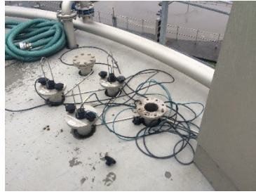
Cleaning of the N 2 O Wastewater Sensor on top of the reject water tank at VandCenterSyd, Odense, Denmark
