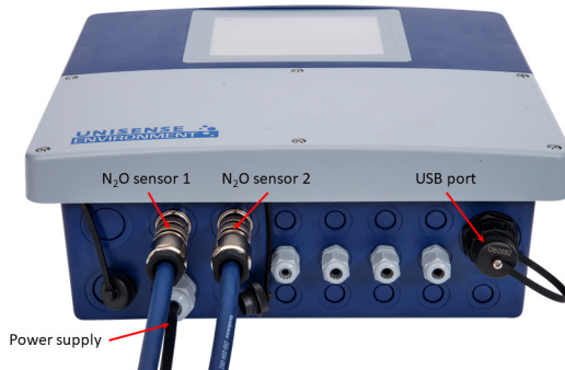
Back view of the N 2 O Wastewater Controller showing connections.
